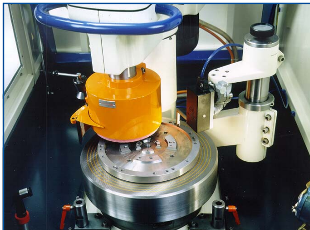
Grinding area with measuring gauge*
